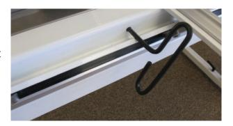
10. With the power cable unplugged and the motors in the engaged position (use the manual engagement/disengagement tool if necessary), ensure that as the quilting machine is moved in both the X and the Y directions, the corresponding gears are rotating, as well.
