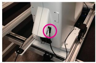
Plug the end of the carriage encoder cable
