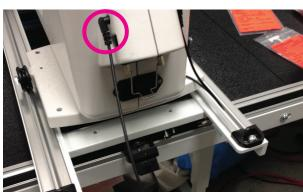
Plug the small end of the Pro-Stitcher carriage communication cable (see Parts List, item M) into the top right connector, labeled Pro-Stitcher, on the machine back connection panel.
