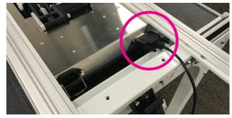
6. Plug the 12' power cord (see Parts List, item I) into the back of the Pro-Stitcher carriage. Secure the power cord into the Pro-Stitcher carriage by pressing the wire cord-retaine onto the cord.
