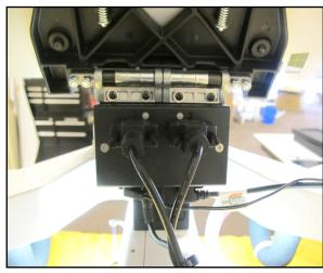
36. Remove the computer from its packaging. Lift up slightly on the center of the top bracket and install the computer into the computer bracket by sliding it into the black bracket from the side until it is centered.
