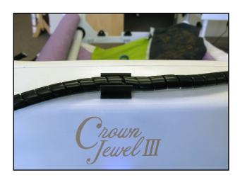
28. The small black cable with the black 3-connector clip should be routed underneath the P-Pod and snapped into the quilting machine's Y-encoder.
