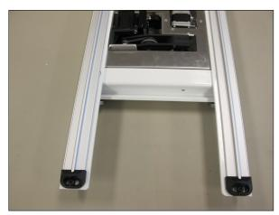
7. Place the Pro-Stitcher carriage on the frame. Starting at one end of the table, begin mounting the blue Flexirack to the front of the table while aligning it to the front white gear on the carriage.
