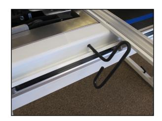
30. With the power cable unplugged and the motors in the engaged position (use the manual engagement/disengagement tool if necessary), ensure that as the quilting machine is moved in both the X and the Y directions, the corresponding gears are rotating as well.
