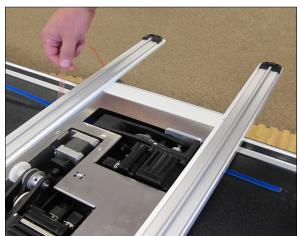
8. Use the carriage as a guide and align the blue Flexirack with the white gear along the length of the table (see arrow at right), removing the pink protective layer and pressing downward on the blue Flexirack while moving down the entire length of the table.
