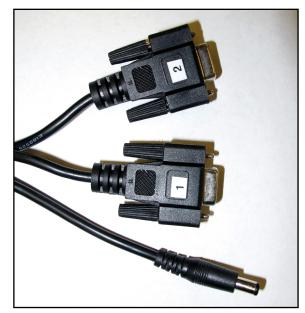
Insert the barrel connector into the center jack located on the bottom edge of the black box that is mounted to the back of the computer bracket. Attach the two 9-pin serial cables to the appropriate ports on the back of the same box, making sure cable connectors are plugged into their corresponding ports on the black box.
