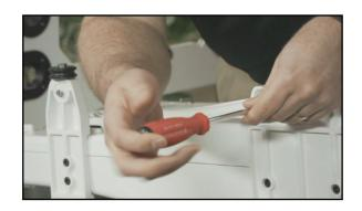
13. Attach the Y-Rack to the bottom of the front and rear base plates. The blue Flexirack should be toward the middle of the machine while the bolt holes should be toward the outside. Use the screws that were removed from the front and rear base plates (or use the two smallest screws in the Base Plate Repair Kit [see Parts List, item D] if your machine had no screws here).
