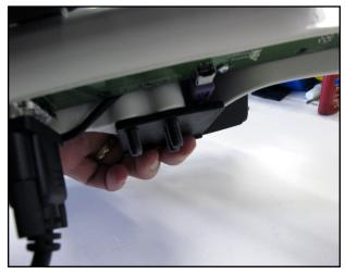
33. Position the handlebar over the computer bracket such that the screws go through the three holes in the bracket.
