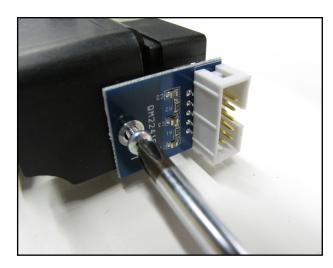
17. Gently pull the circuit board outward toward the front of the quilting machine (the same direction the screw came out).
