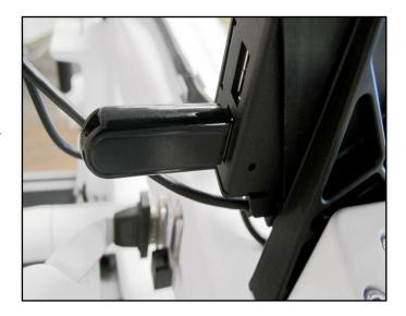
**■ IMPORTANT:** It is not necessary to power down Pro-Stitcher to install or remove the USB flash drive, but take care not to remove the flash drive while the system is saving to or loading from the drive.
