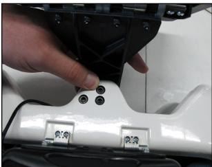
34. Secure the handlebar and bracket in place on the machine head using the three handlebar bolts.
