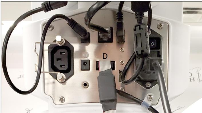
15. Attach the 12A power cord to the inlet at the back left of the carriage (A). Use the wire bale to hold the cable in place (B). Plug the opposite end of the power cable into a wall outlet or other appropriate power source.
