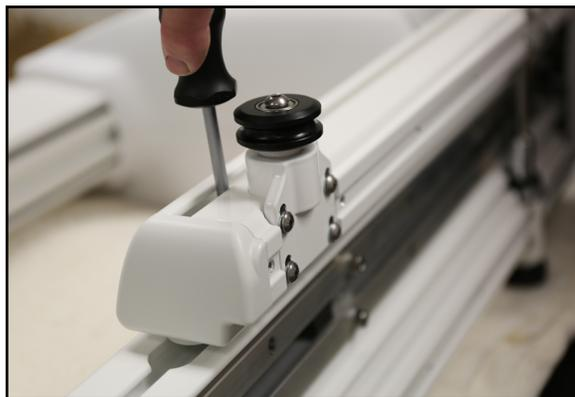
2. Remove the screw, washer, and T-nut from the placeholder end cap.
