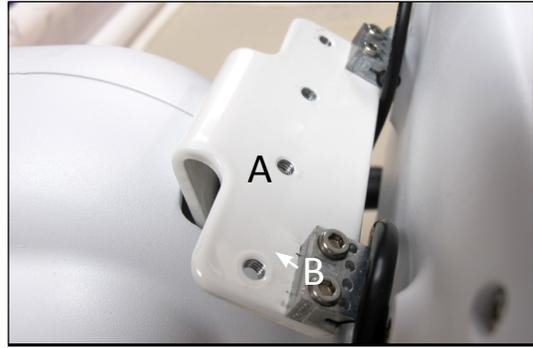
2. Attach the Pro-Stitcher computer bracket (see *Parts List, item E*) by aligning the four holes in the bracket with the four holes along the top of the display bracket.
