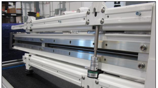
8. Attach the Y-rack black rack (see *Parts List, item F-2*): Slide the notched end into the end cap and line up the three keyholes in the black rack with the three low-profile screws from step 7.
