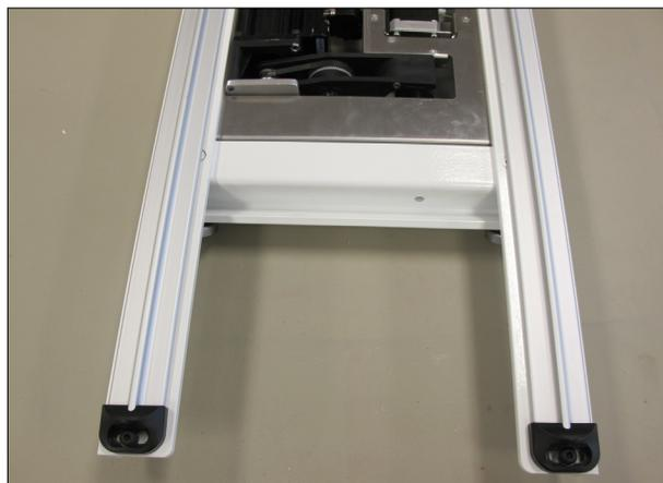
2. Place the Pro-Stitcher carriage on the frame. Starting at one end of the table, begin mounting the blue Flexirack to the front of the table while aligning it to the front white gear on the carriage.
