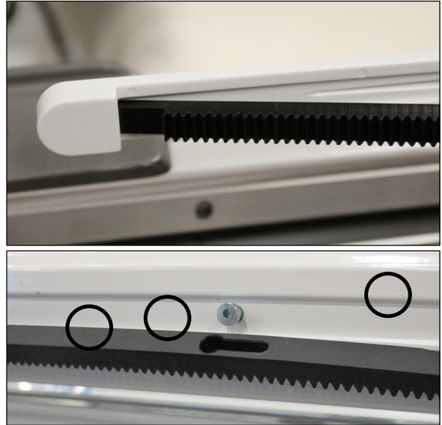
9. Slip the keyholes in the black rack onto each screw, beginning with the screw closest to the front of the machine.
