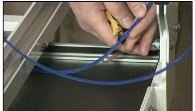
6. At both ends of the blue Flexirack, use two of the small metal clamps (see *Parts List, item B*) to hold the ends firmly in place. The clamps have a hole through the center and a lip on one end. The lip should be on the side opposite the blue Flexirack. Place the clamps where they will be attached and drill pilot holes using the 3/32-inch drill bit and then use a Phillips screwdriver to fasten the clamps on both sides of the Flexirack to the table.
