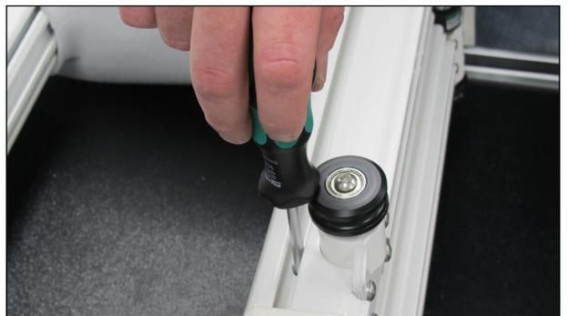
7. Insert three M4 x 12 socket-cap low-profile screws -- one into each of the three holes indicated in the photo. Partially tighten them, leaving them about 1/4 inch out.
