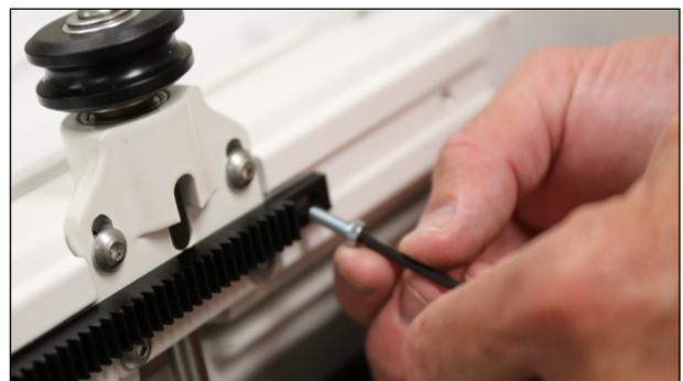
12. Turn the Infinity upright and place it on the Pro-Stitcher EZ Carriage. Ensure that the white Y-rack gear engages with the black Y-rack. You may need to manually engage the EZ carriage using the manual engagement tool provided.
