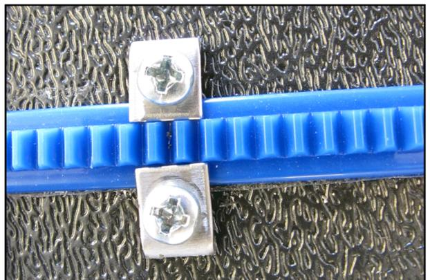
△ **CAUTION:** Do not use the larger drill bit included in the emergency repair kit, as this is the wrong size for the Flexirack clamps.
