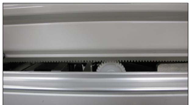
13. Inspect the machine and carriage to ensure that all four machine wheels are lined up and touching the aluminum carriage tracks and that the wheels and the carriage track are clean and free of any dust or debris.
