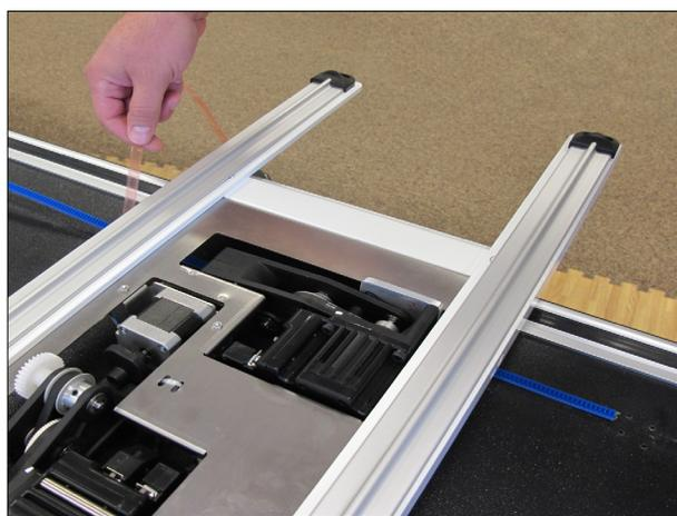
3. Use the carriage as a guide and align the blue Flexirack with the white gear along the length of the table (see arrow at right), removing the pink protective layer and pressing downward on the blue Flexirack while moving down the entire length of the table.
