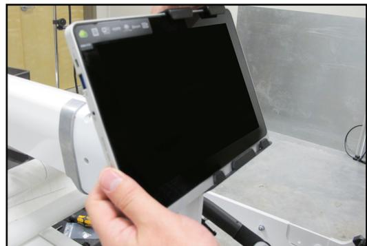
5. Locate the USB cable provided with Pro-Stitcher (see *Parts List, item K*). Connect one end to the USB port on the tablet computer and the other end to the USB port on the side of the Infinity.
