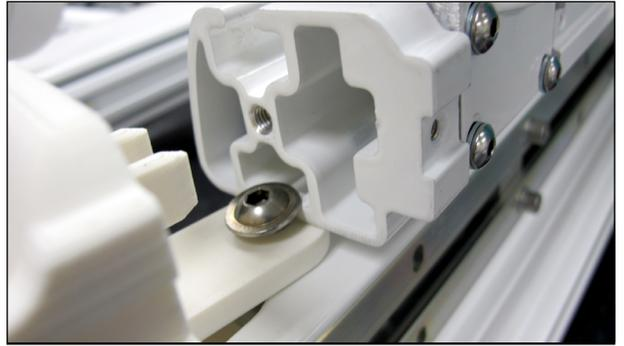
5. Use the provided M6x16 screw and tighten the front screw of the Y-rack end cap with the 5mm hex wrench.
