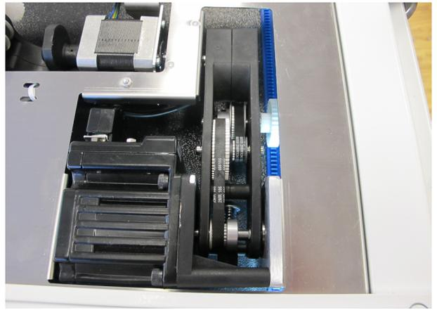
4. Double check the alignment of the carriage white gear with the blue Flexirack by rolling the carriage along the entire length of the table.
