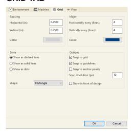
In this section you can set the parameters for the grid by selecting Spacing for both the Horizontal and Vertical. Other options available include choosing colors for both the spacing options and the Major grid lines.
