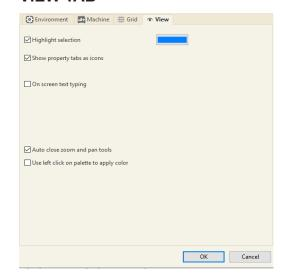
View in this section, choose the color a design element will display when you select it in the software. You can also choose to enable on screen text typing, auto close zoom and pan tools and use the left click on palette to apply color.
