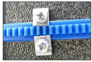
NOTE: As an alternative, use one clamp at each end. Slide the lip of the clamp over the last tooth of the blue Flexirack, drill a pilot hole, and screw in place.
