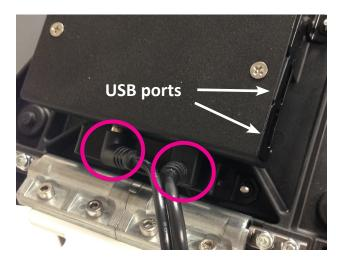
■ IMPORTANT: The tablet shown is the Acer Switch Alpha 12 series tablet. Your tablet may be a different make or model. Connect the USB and power cables in their proper location based on your make and model of tablet. Do not confuse the audio port with the power port (they are often similar in size but are usually marked with headphones for the audio port and a DC electrical symbol for the power port).
