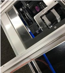
3. Use the carriage as a guide and align the blue Flexirack with the white gear along the length of the table (see arrow at right), removing the pink protective layer and pressing downward on the blue Flexirack while moving the carriage down the entire length of the table.
