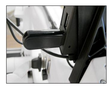
■ IMPORTANT: It is not necessary to power down Pro-Stitcher to install or remove the USB flash drive, but take care not to remove the flash drive while the system is saving to or loading from the drive.
