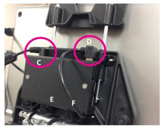
4. The open USB ports on the black box are for the USB Flash drive to load designs or update the software, or for plugging in a keyboard or mouse.
