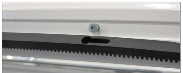
9. Slip the keyholes in the black rack onto each screw, beginning with the screw closest to the front of the machine.
