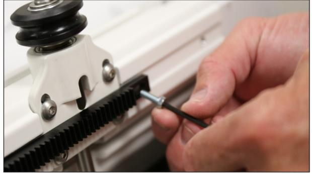
12. Turn the Infinity upright and place it on on the Pro-Stitcher EZ Carriage. Ensure that the white Y-rack gear engages with the black Y-rack. You may need to manually engage the EZ carriage using the manual engagement tool provided.
