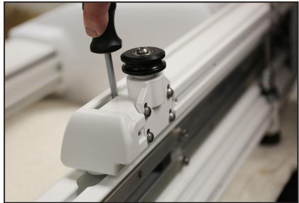
2. Remove the screw, washer, and T-nut from the placeholder end cap.
