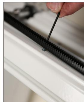
11. Tighten the fourth screw in the slot at the back end of the black rack.
